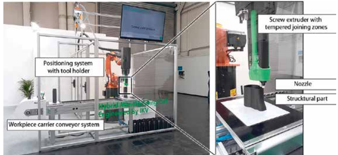
Fig. 1. IKV's hybrid production cell in live operation at the Hanover Fair 2018, as it produces a structural part at a production speed of 6g/min (© IKV)
