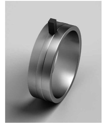
Fig. 6: Schematic diagram of block-on-ring wear measurement
