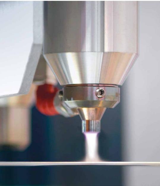
Preparation for the hybrid injection moulding process: functional coating with PlasmaPlus®
