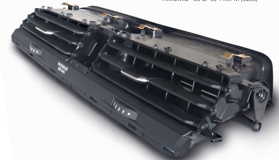
Air discharge installation VW Touran: AKROMID® B3 GF 60 4 RM-M (5238)
