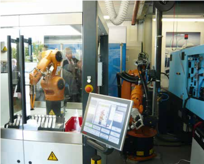
Fig. 2. Profile of the pilot plant. The metal test specimen is picked up by the robot (left), cleaned, then surface-coated with plasma. After this, a second handling system takes over (center), the test specimen is heated to more than 220°C and is placed in the mold (right). There, the plasma-pretreated insert is overmolded with polyamide (© Hanser/F. Gründel)
