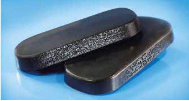
Fig. 1. Effect of increasing heterogeneous nucleation (upper component: nucleated, lower component: not nucleated)
