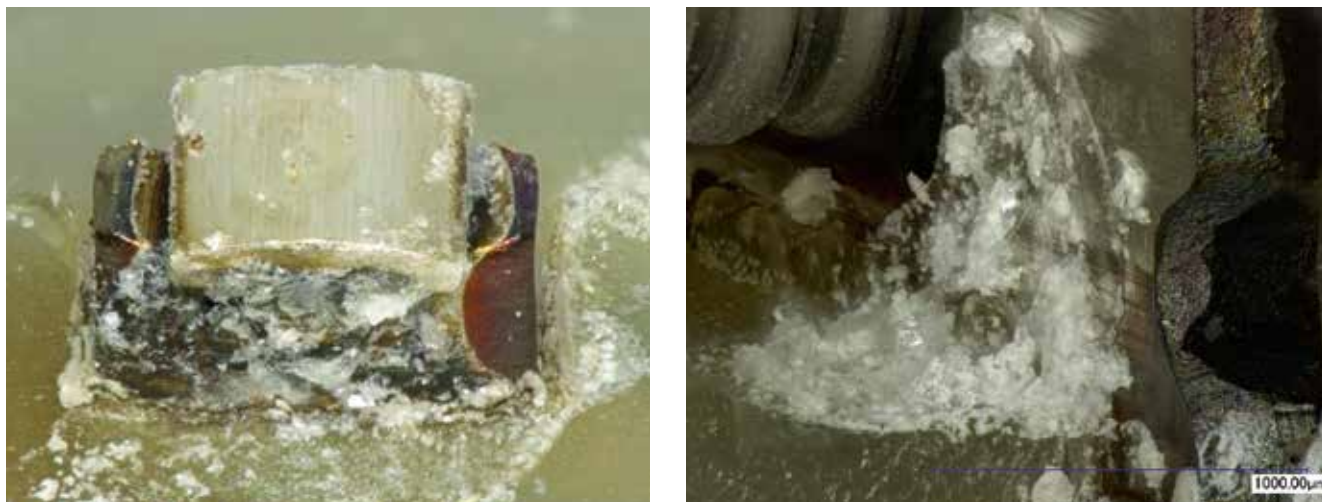
Fig. 3. Metal soap deposits (left), and a detailed image of the deposits (right)
