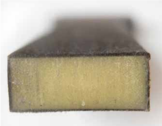
Fig. 3. Tensile test bar made from Akromid C3 GF 30 5 XTC natural (4499) after 1,000 h at 210 °C (© Akro-Plastic)
