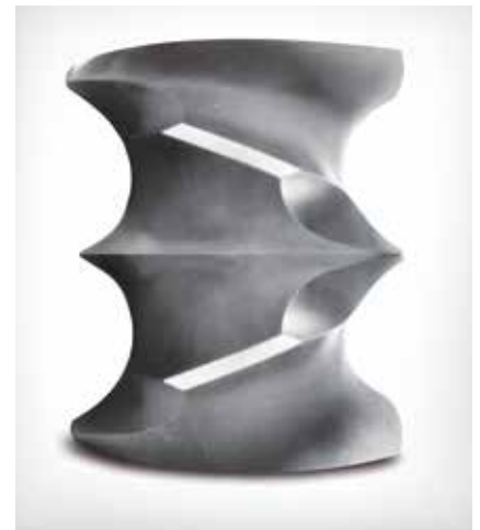
Fig. 3. Mixing element in a kneading block-free screw for the production of biobased masterbatches at low temperature
